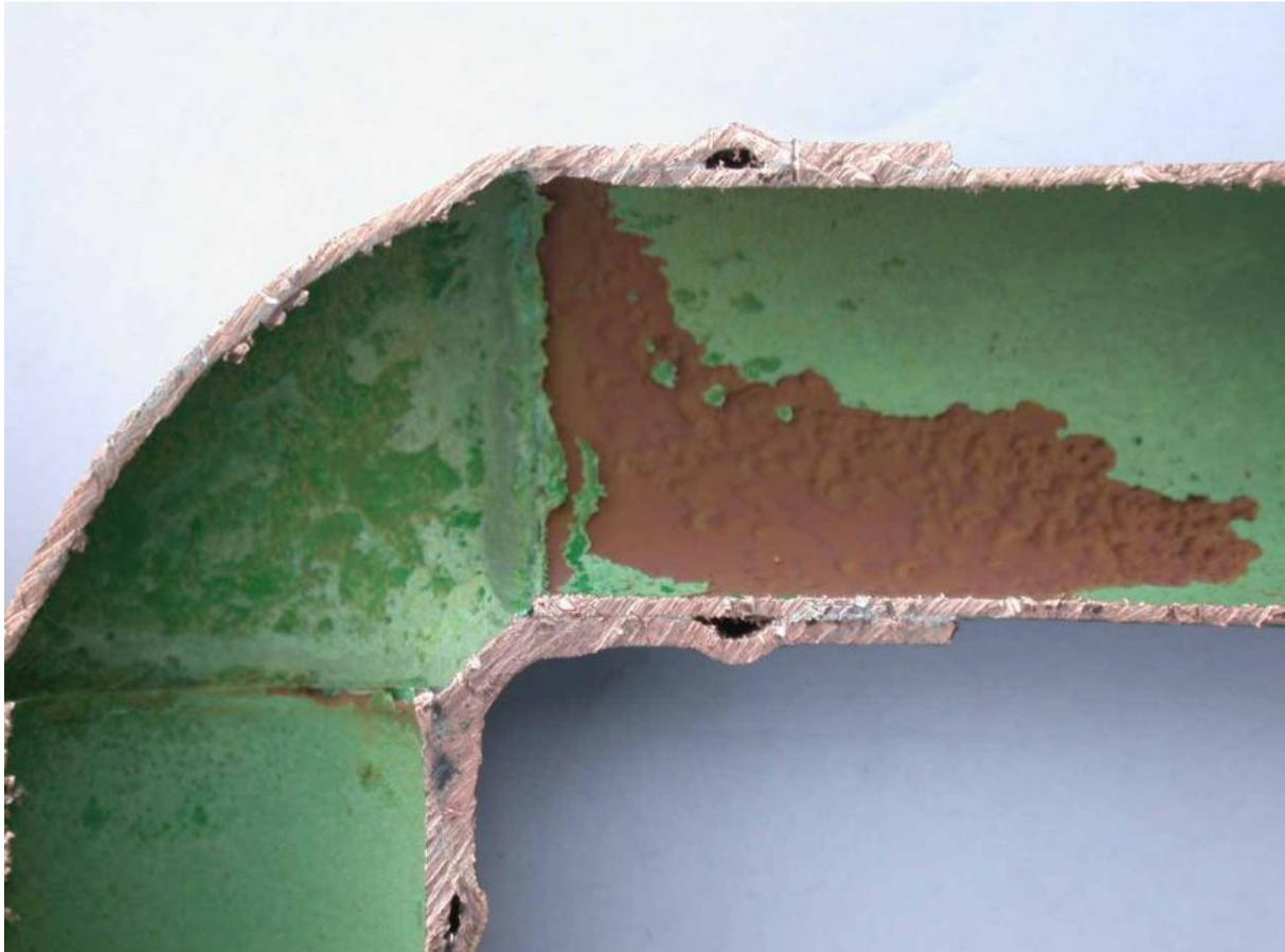
*Figure 4 Erosion Corrosion at elbow.*
