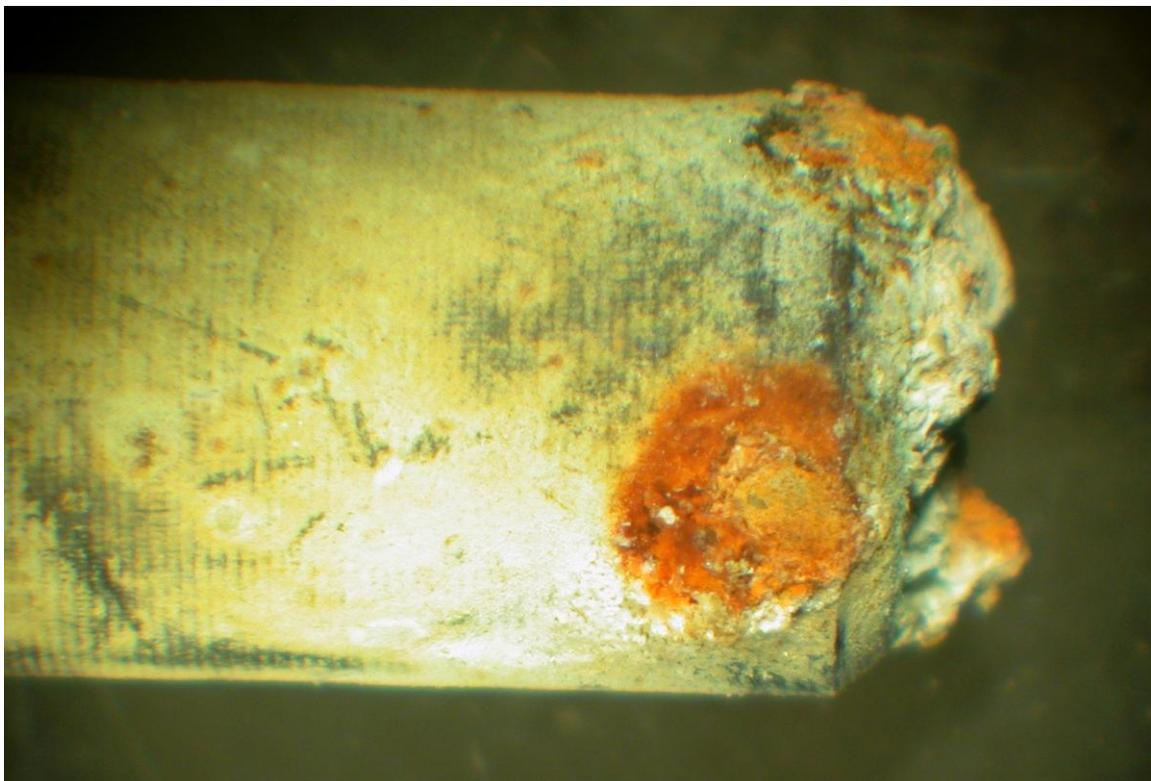
Figure 6 Dezincification of a temperature probe.
