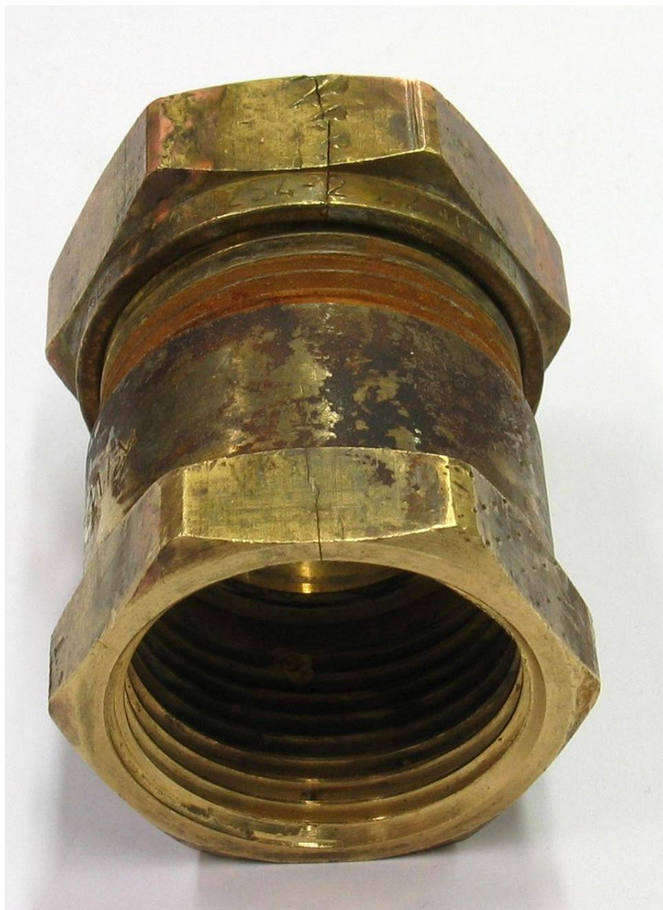
*Figure 7 Stress corrosion cracking in a brass fitting.*
