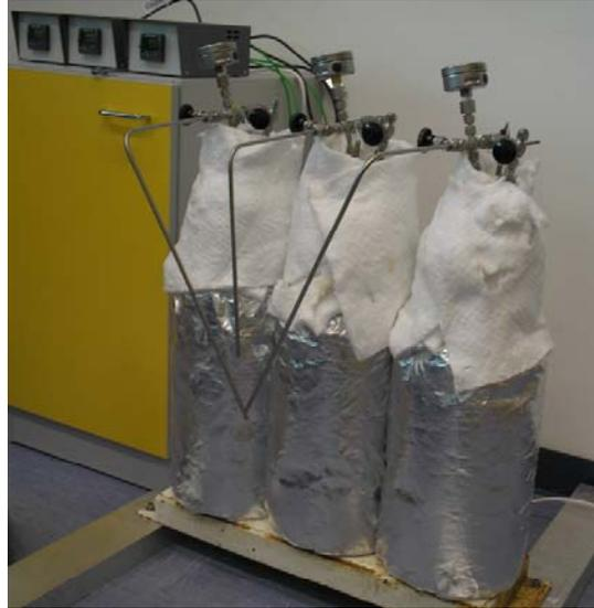
**Figure 7: Autoclave vessels used for conditioning specimens at elevated pressure**
