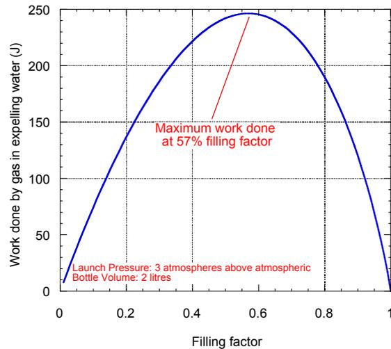
As the filling factor is reduced, i.e. as we reduce the amount of water in the bottle (and increase the volume of air), the stored energy increases because the volume of gas increases. The peak arises because the work that the gas does in pushing the water out of the bottle depends on the gas *expanding*. If the bottle is full of air, then it cannot do much work before all the water is expelled.
