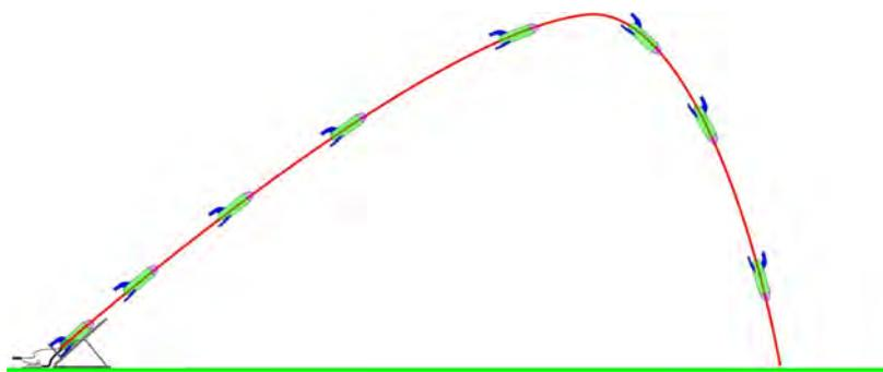
An aerodynamically unstable rocket may start out with its nose first, but its flight will quickly become unstable and it will flap and tumble in the air, and then simply fall to Earth.
