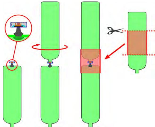
The last step is to add a fairing to reduce drag. One clever way to do this is to cut out the central part of yet another bottle and slip it over the combined bottles.
