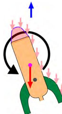
For *Rocket B* (right) the centre of mass lies further backwards along the rocket axis than the centre of pressure. The extra drag forces therefore act more on the front end of the rocket and tend to ‘push it even further out of line’.
