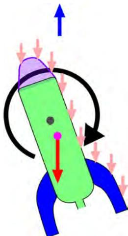
For *Rocket A* (left) the centre of mass lies further forwards along the rocket axis than the centre of pressure. The extra drag forces therefore act more on the back end of the rocket and tend to ‘push it back into line’. Technically we say the drag forces exert a torque which acts about the centre of mass to restore optimal flight attitude.
