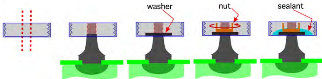
To do this one first places a rubber washer over the valve stem, and squeezes it tightly into place with a nut made from a cut down cap for a tyre valve. One then seals the entire connection with silicone sealant and allows the assembly to set for 24 hours.
