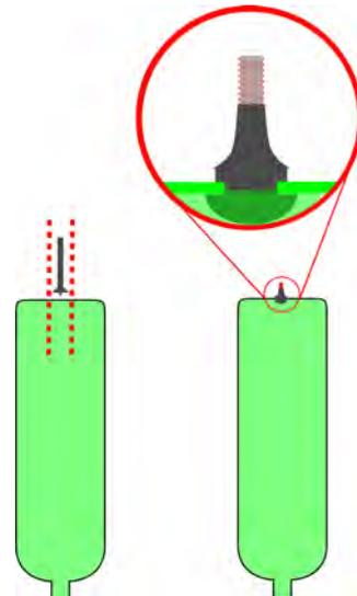
Now we need to attach another bottle to this valve. To do this we begin with a standard bottle cap and drill a hole which will allow the stem of the tyre valve to protrude as shown below. We now have to make the connection pressure tight.
