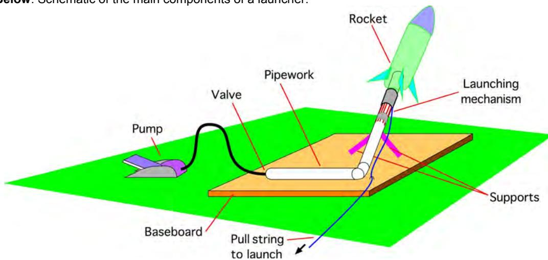
**Below Left :** A typical rocket launcher without a launch tube: we'll call this Design A.
