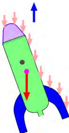
The forces along each portion of the rocket are difficult to calculate or measure precisely, but there will be some point on the rocket which is their effective point of action. This point is known as the *centre of pressure*, and is marked with a purple dot in the figures right and left.
