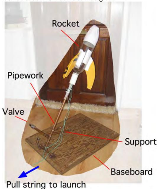
**Below Right :** A typical rocket launcher with a launch tube: we'll call this Design B.
