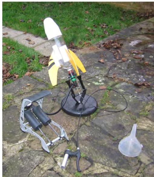
**Far Right:** Filling the rocket with a measured charge of water.
