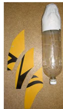
Corrugated cardboard will do, but does tend to go soggy after a few launches. Also many packaging materials have the same design requirements as water rocket fins (high rigidity-to-weight ratio). One common choice is to cut up old CD's to use as fins. If you do this please then make sure you put tape over any sharp edges in case your rocket should hit someone.
