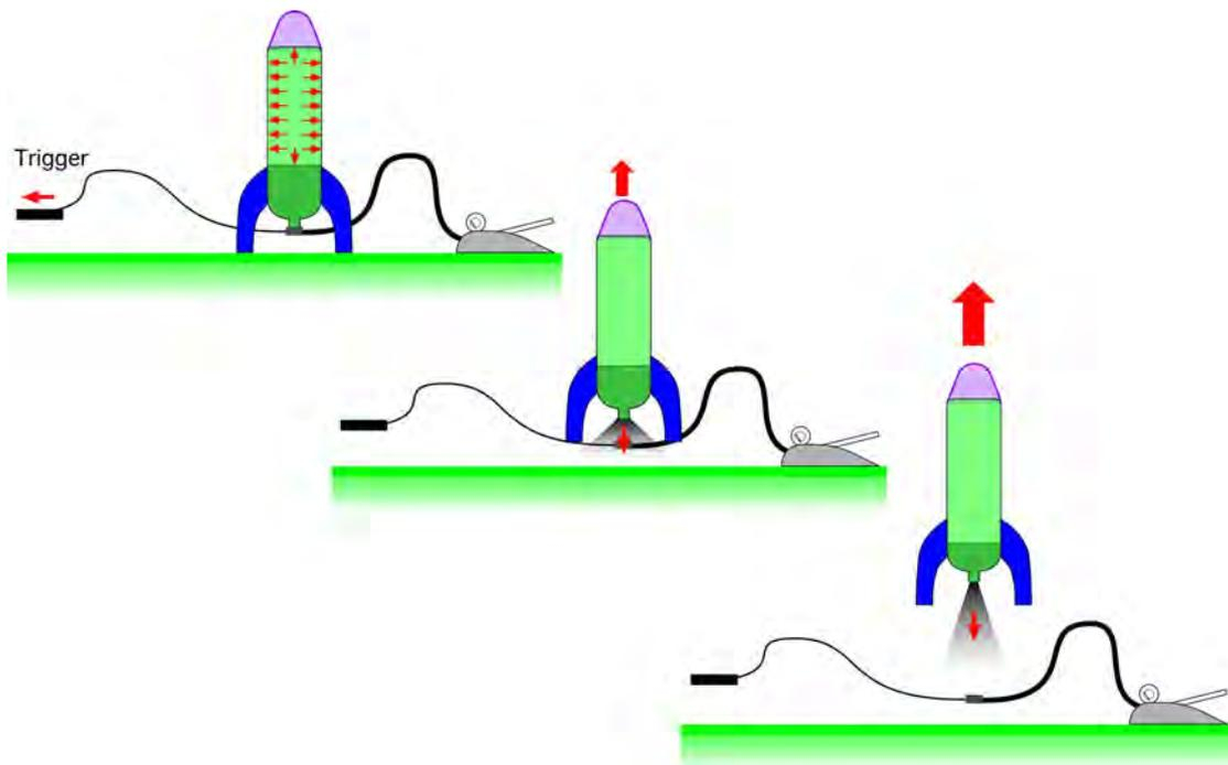
Peak launch velocities can easily reach 30 metres per seconds (about 60 miles per hour), and without too much difficulty its possible for a rocket to reach heights in excess of 30 m. But launching a rocket straight up in the air can be dangerous...
