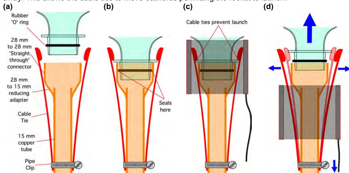
The major problem with Design A is that the rocket is only supported at the neck, and since a large rocket can weigh several kilograms when filled with water, this makes the rocket liable to 'sag' before launch. This could be overcome by the addition of either a launch ramp to support the rocket, or a launch tube. A photograph of the launcher in action can be seen in the collection on Page 5 (one down from the top right), where Jaco has used an improvised launch ramp.
