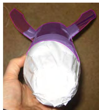
**Right:** In this attitude, additional surfaces (outlined and shaded) are exposed to the oncoming air. Some of these surfaces are on the side of the rocket and some are on the fins.
