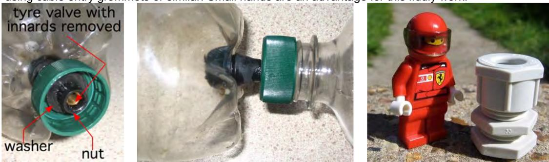
**Alternative technique:** Using similar principles to those described above, a cable entry grommet for electrical wiring (above right) can be used to make a large aperture bottle connector.
