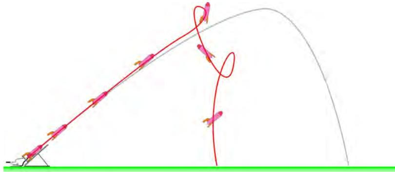
In order to make your rocket fly 'like a rocket' rather than 'like a bottle', the weight needs to be in the front half of the rocket. However depending on the design of your fins, this may or may not be enough to ensure aerodynamically stable flight. One of the most important properties of your rocket is the position of its *centre of mass*, sometimes called its *centre of gravity*.
