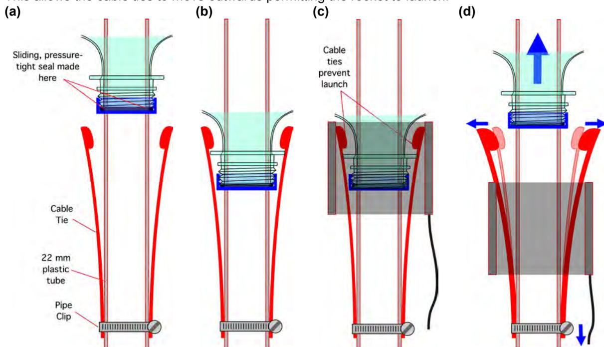
Designs A and B both use cable ties as a key component in the launching mechanism, but as the photographs below show, they adopt a what I can only describe as different design philosophies. Dave has gone for the *minimum* of three cable ties, and Jaco has gone for the *maximum* number of cable ties that can be arranged around the rim of the bottle. Which is better? I don't know: they both work very reliably!
