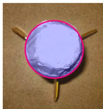
**Right:** Exposed surfaces of the rocket: The circle shows the area of the rocket exposed to the oncoming air. The fins are rather thin and move easily through the air.
