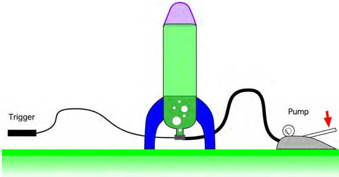
When the trigger activates the release mechanism, the pressurised air within the rocket pushes the water rapidly out through the nozzle, sending the rocket rapidly into the air.
