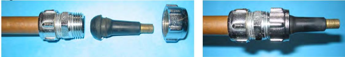
A similar arrangement can be made with 22 mm plumbing fittings, but there it will be necessary to drill a hole in an end-cap, and to fit the car tyre valve in place. Glue or sealant should not be necessary, because the tyre valve fitting is designed so that as the pressure increases, the seal will improve. A similar design can also be made using bicycle tyre valves
