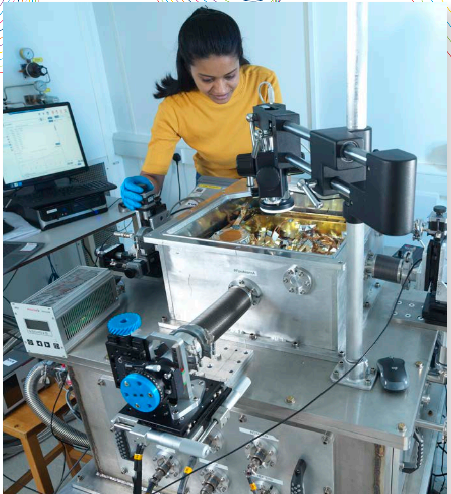
NPL scientist preparing the cryogenic probe station at the SuperFab for automated electrical characterisation of devices at 4 K.
