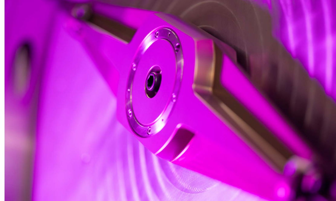
Water droplet erosion: Designed and built by NPL the water droplet erosion facility is capable of accelerated testing at speeds exceeding 300 m/s.
