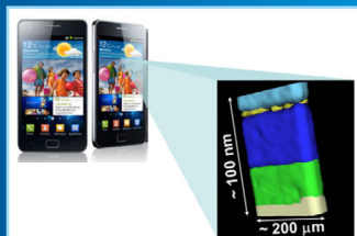
3D SIMS image of one pixel in an OLED display
