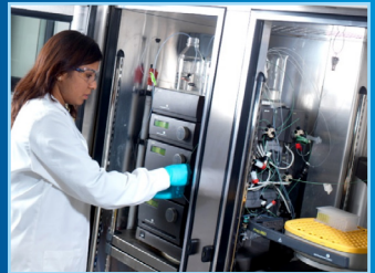
AKTA purification system for protein and DNA separation and analysis
