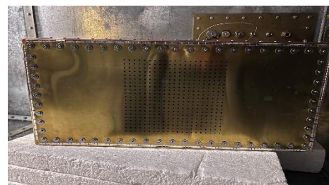
Figure 2. The enclosure and the aperture comprising an array of circular holes – the enclosure's dimension is 300×500×600 (mm)
