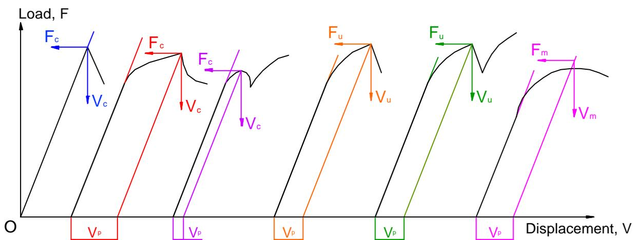
*Figure A1. Definition of F (F<sub>c</sub>, F<sub>u</sub> or F<sub>m</sub>) and V<sub>P</sub>*
