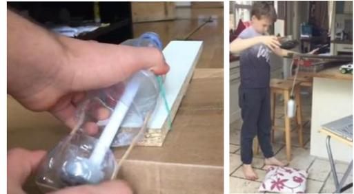
**Jack** the brilliant idea of using a dropping weight (water bottle) to provide a consistent force.
