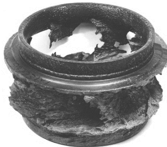
Figure 3: Erosion of grey cast iron impeller after two months handling coal dust.
