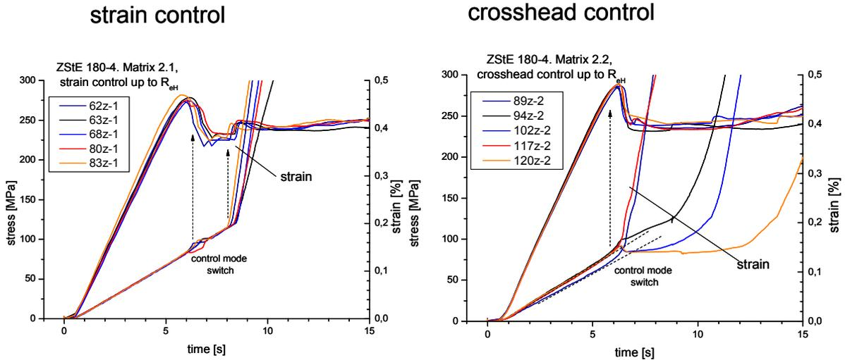
Figure 43: Stress, strain vs. time for ZStE180, mode 2.1 and 2.2
