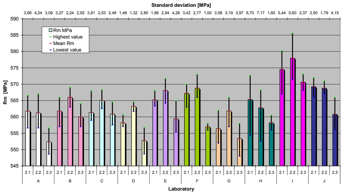
Figure 32:  $R_m$  for material S355 with test pieces ISO12.5x50 and extracted outliers
