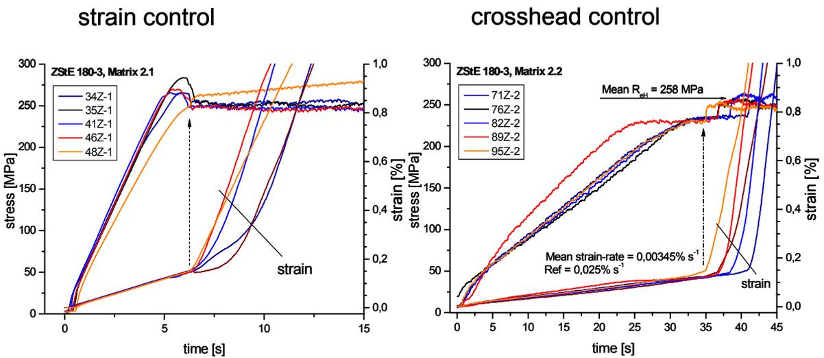
Figure 44: Stress, strain vs. time for ZStE180, mode 2.1 and 2.2
