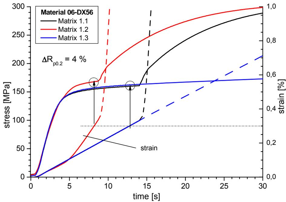
Matrix 1.2 with const. crosshead separation rate:  $v_c = L_c \times \dot{\epsilon}_{Lc}$
