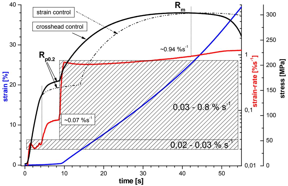
Figure 41: Stress, strain and strain rate vs. time for DX56 (ISO20x80) for modes 1.1 and 1.2 and the allowed testing speed
