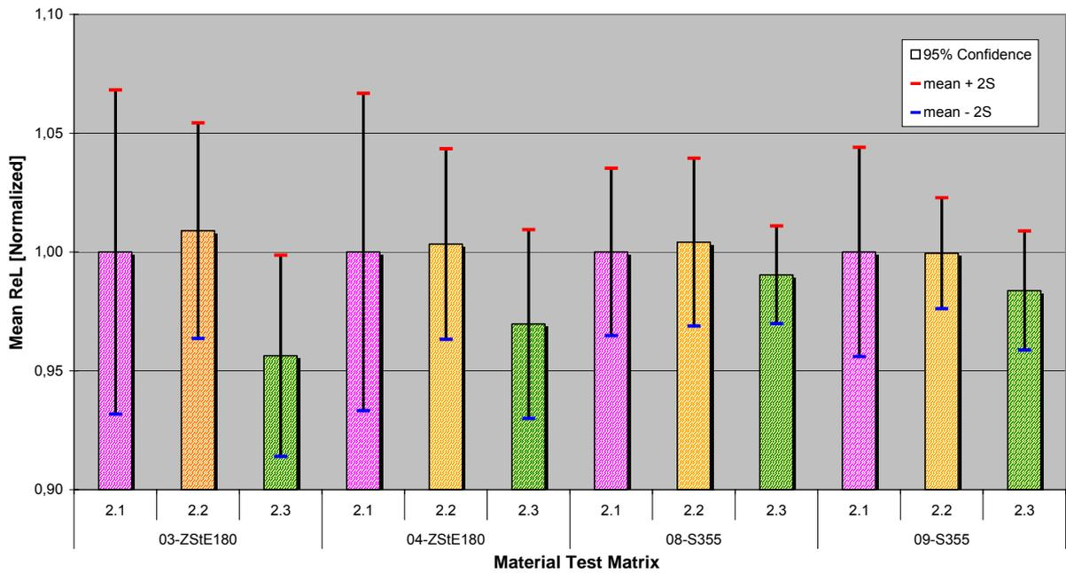
Figure 35: Normalised test results for  $R_{eL}$  of the materials ZStE180 and S355
