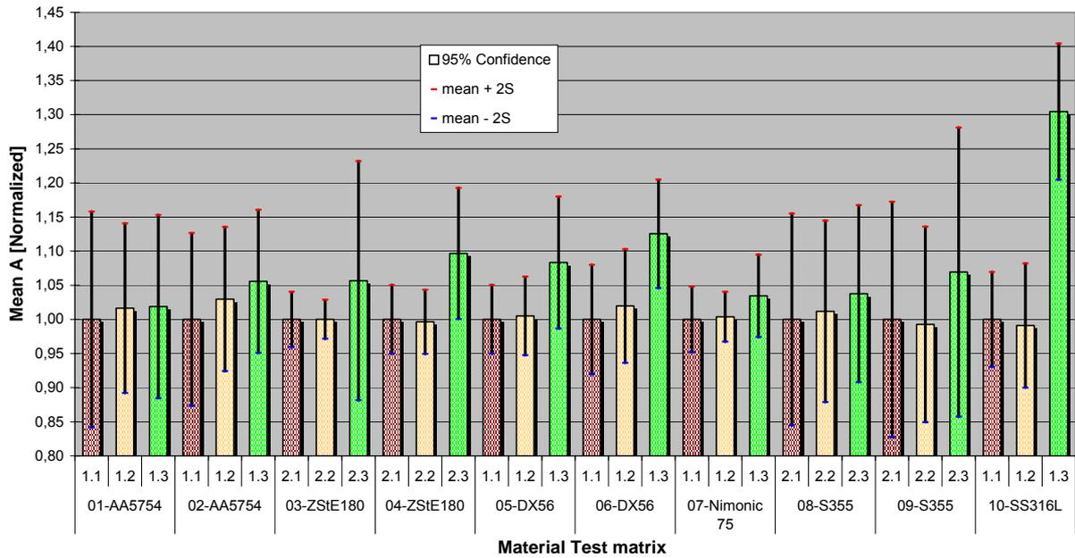
Figure 37: Normalised test results for A of the materials AA5754, ZStE180, DX56, Nimonic 75, S355 and SS316L
