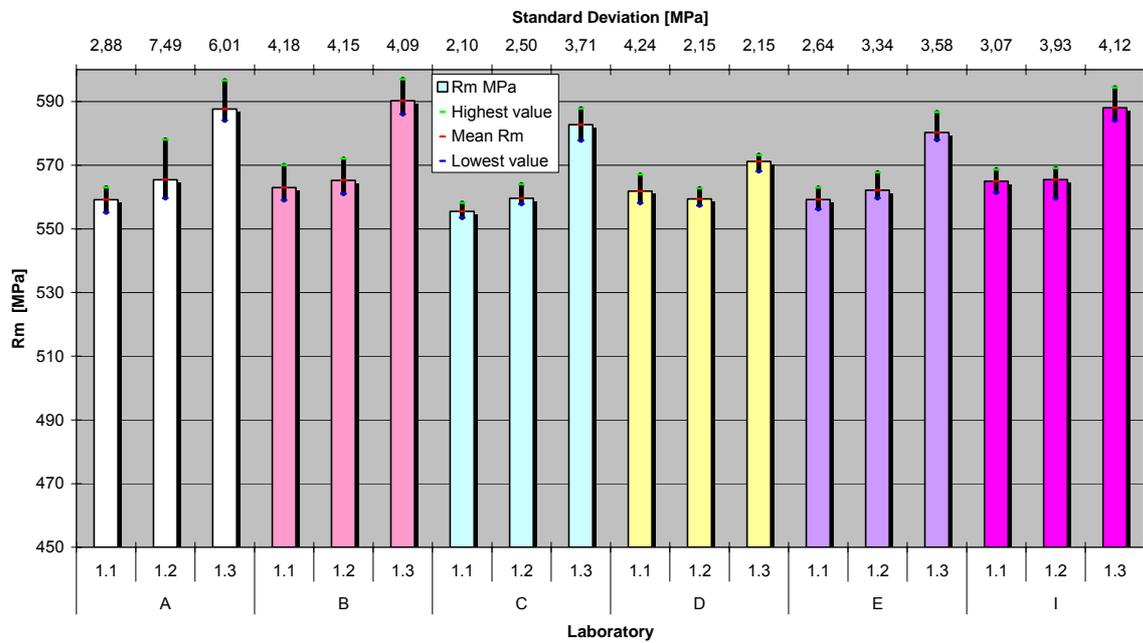
Figure 14:  $R_m$  for material 316L with test pieces M16-10x50 and extracted outliers
