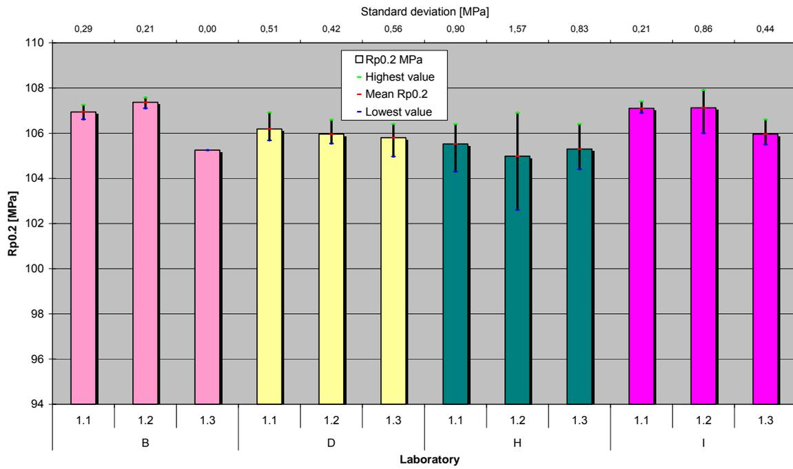
Figure 17:  $R_{p0.2}$  for material AA5754 with test pieces ISO12.5x50 and extracted outliers
