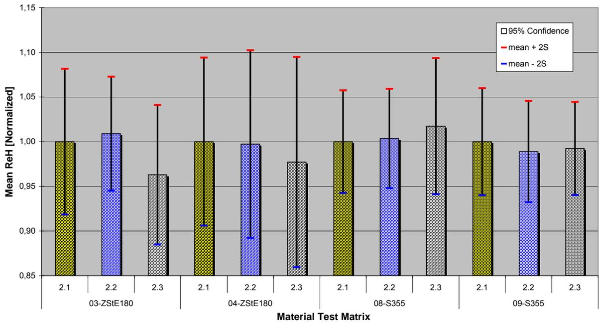
Figure 34: Normalised test results for  $R_{eH}$  of the materials ZStE180 and S355
