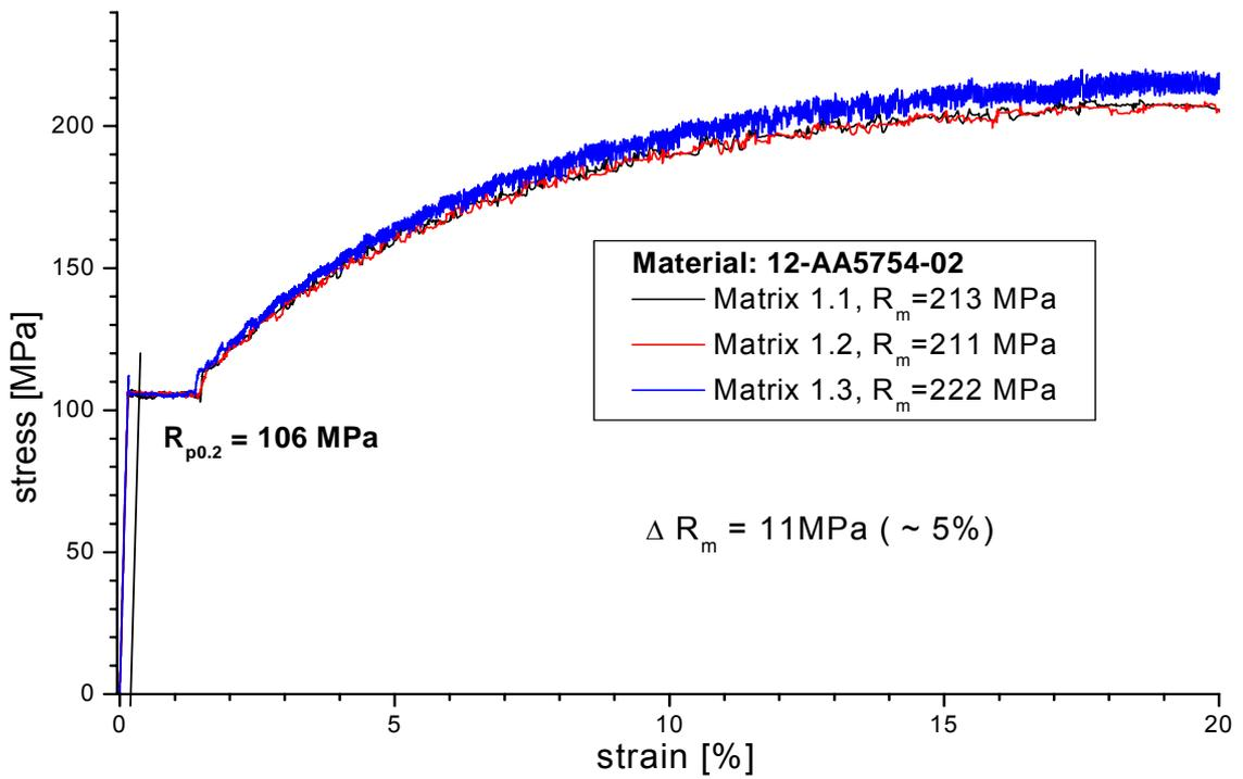
Figure 42: Stress strain curves for AA5754 (ISO20x80) for modes 1.1, 1.2 and 1.3
