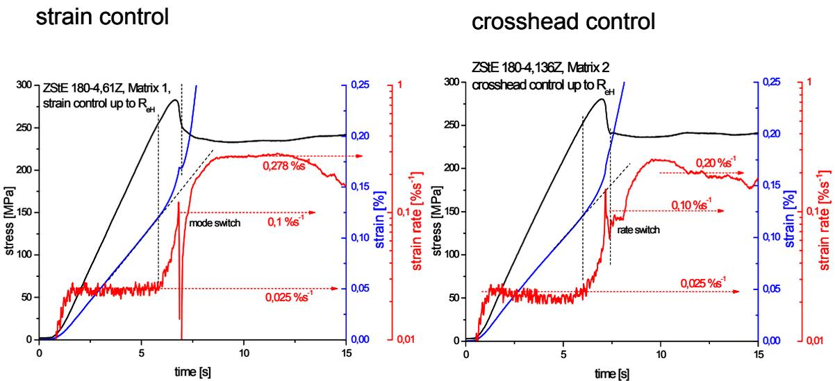
Figure 45: Stress, strain, strain rate vs. time for ZStE180, mode 2.1 and 2.2
