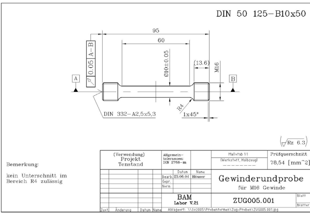
Figure 4: Test piece geometry according to DIN 50125 for cylindrical threaded samples of S355 and 316L
