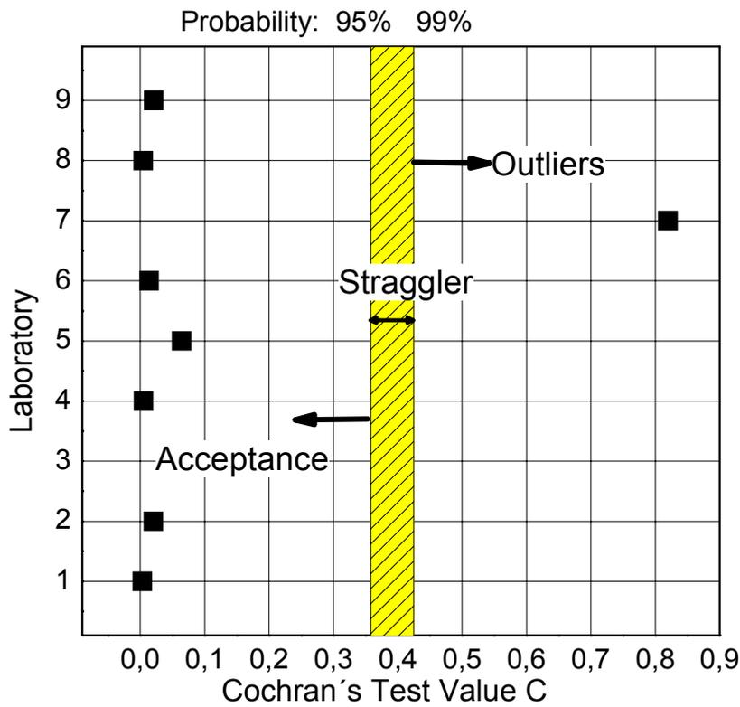
Figure 8: Cochran test for the determination of an outlier
