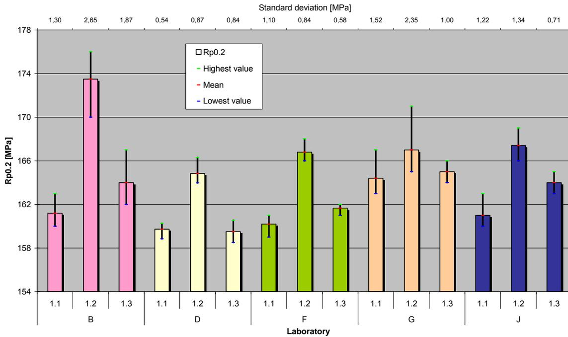
Figure 10:  $R_{p0.2}$  for material DX56 with ISO 20x80 test pieces and extracted outliers
