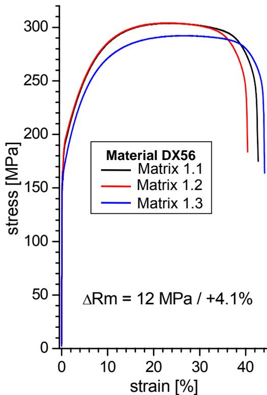
Figure 40: Stress strain curves for modes 1.1, 1.2, and 1.3 at the material DX56
