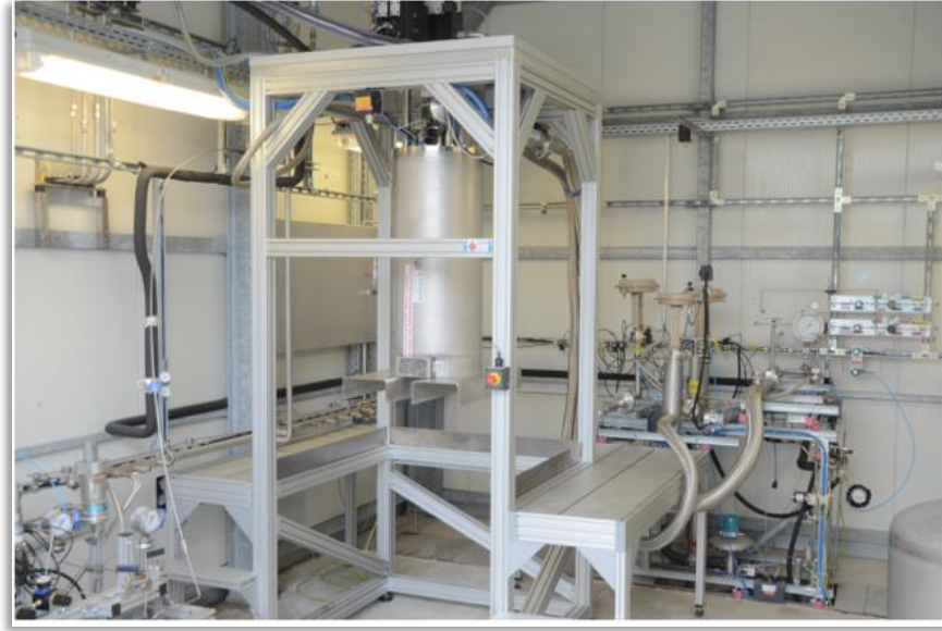
Figure 5 Liquid hydrogen testing machine at EnergieTechnologie.
