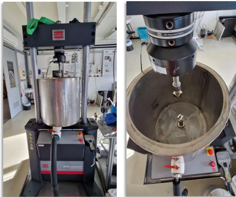
Figure 3 In-situ LN 2 test setup MTS100 at Karlsruhe Institute of Technology.
