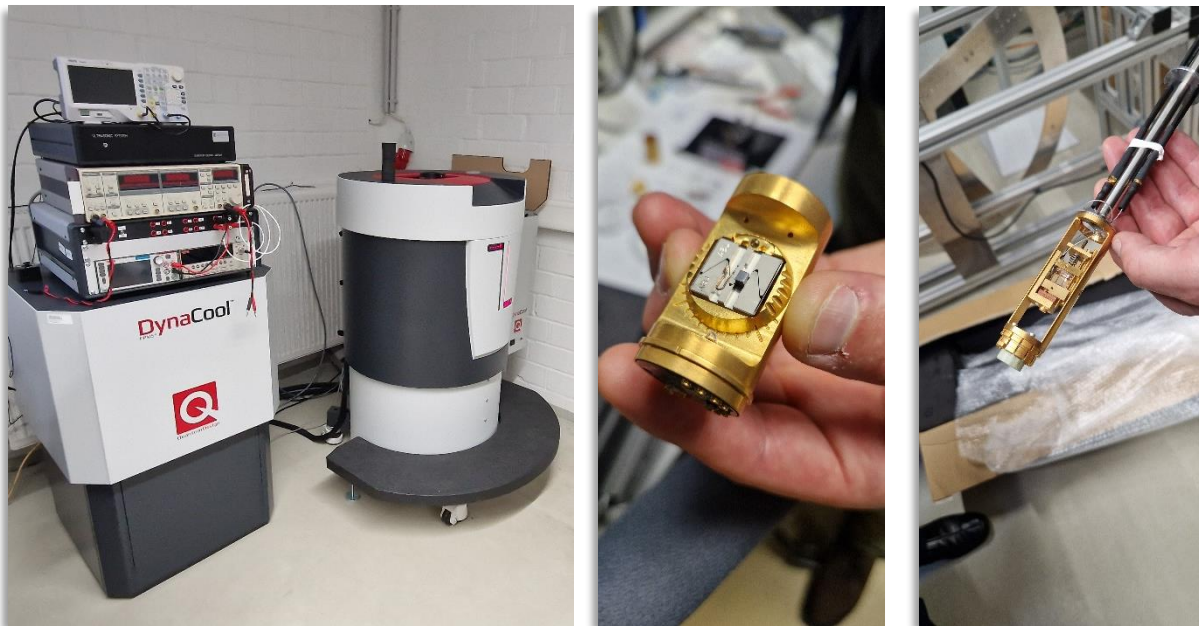
Figure 4 Quantum Design Physical Property Measurement System with thermal property probes.
