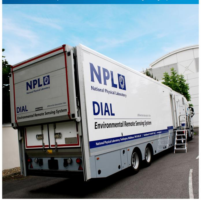
The DIAL system is able to monitor atmospheric pollutants remotely, at ranges of up to 1 km. DIAL measurements are real-time, directly traceable to primary standards of gas concentration and are free from interference and contamination. DIAL is particularly useful for measurements of emissions from process areas, tanks, flares and diffuse sources, e.g. landfill sites (Innocenti et al., Remote Sensing 2017, 9, 953; Innocenti et al., Remote Sensing 2022, 14, 4291).
