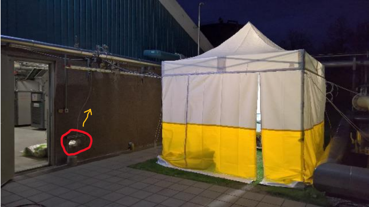
Figure 1: Measurement campaign at Ribe Biogas (Nov. 2024). The opened building door separates ATEX (inside) and non-ATEX (outside) areas where the tent was set up. The biomethane was taken via a PTFE tubing (marked yellow arrow) from the ATEX area to the analysers in the tent through an opening in the wall (marked in red). Several indoor/outdoor gas in-take points were available in the vicinity of the tent.
