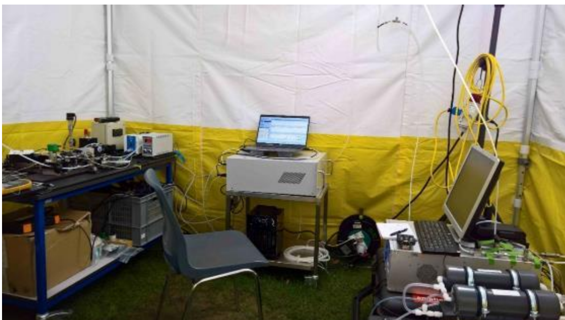
Figure 11: Far-UV (left), MAX-iR (middle) and OF-CEAS/OGS (right) analysers in the tent in Ribe.
