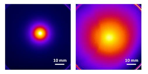
X-ray beam detected on LYSO 100's MeV e-  $\rightarrow$  multi-MeV x-rays
