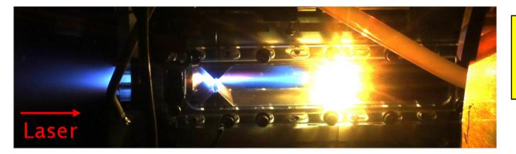
Field strength up to 100 GV/m behind the laser pulse
