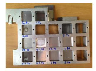
Range of convertors 100µm Al to 5000µm Ta
