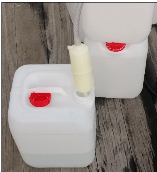
Fig. 3: Direct filtration of the continuously sampled seawater using Pall AcroPak 1500 0,8/0,2 μm filters
