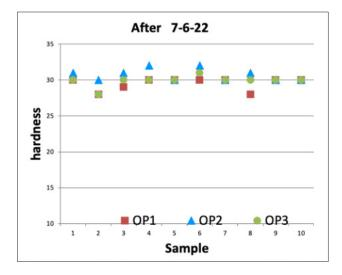
Results of testing by 3 different operators of the same batch of products before and 2 months after the end of the project.
