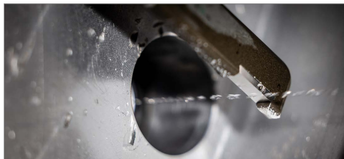
Figure 1: Water droplet erosion: samples located in a high speed rotating arm impact water droplets at speeds in excess of 300 m/s causing erosive wear.
