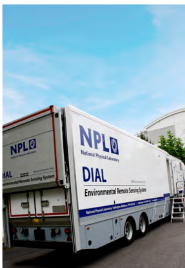
NPL's Differential Absorption Lidar (DIAL), a remote sensing lab-on-wheels, has been used by Defra to provide reliable methane monitoring at landfill sites across the UK.
