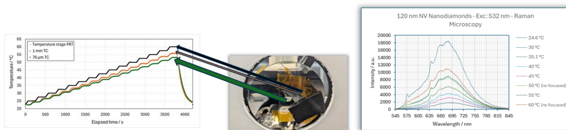
Figure 1. Left. Temperature offset at different positions near the NV diamonds sample in a microscopy stage. Right. Luminescence spectra at different temperature point for 120 nm NV diamonds
