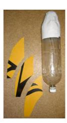
Corrugated cardboard will do, but does tend to go soggy after a few launches. Also many packaging materials have the same design requirements as water rocket fins (high rigidity-to-weight ratio). One common choice is to cut up old CD's to use as fins. If you do this please then make sure you put tape over any sharp edges in case your rocket should hit someone.
