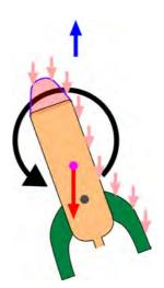
So it is the relative positions of the *centre of mass* and the *centre of pressure* that determines whether a rocket is aerodynamically stable (like *Rocket A*) or unstable (like *Rocket B*). We saw in a previous section how to determine the position of the centre of mass, but how do we determine the position of the centre of pressure?
