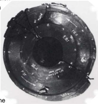
Figure 9. Hinkley Point Failed Disc
