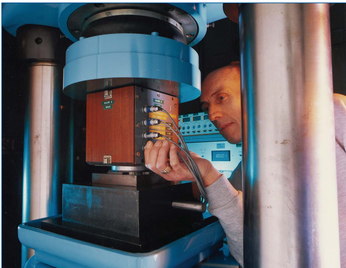
Reference Strain Cylinder Set up in 3MN Strain Cylinder Reference Machine
