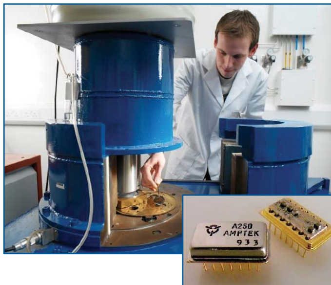
A typical coincidence counter used to standardise radionuclides (insert shows components of a new amplifier system under development)
