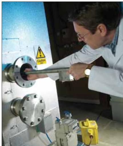
NPL's newly developed 'virtual chimney' which provides a controlled environment where manufacturers can hone their measurement skills and test pollution monitoring equipment over a range of operating conditions.
