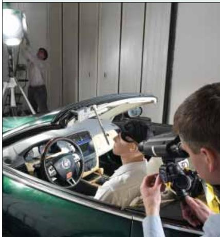
Jaguar Cars Limited are the first company to make full use of our new facilities; NPL scientists have provided valuable feedback on the sunlight legibility of automotive displays. The Ambient Illumination Laboratory (AIL) has been pivotal in creating a method for quantitatively specifying the visual performance of electronic displays that can be easily passed on to suppliers. It also provides the means of establishing fitness for purpose of new display systems.
