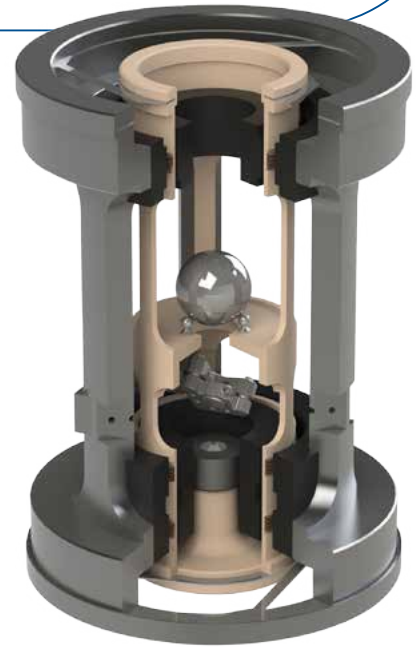
Photo: Concept design for the world's most accurate mass realisation, the NPL next generation Kibble balance
