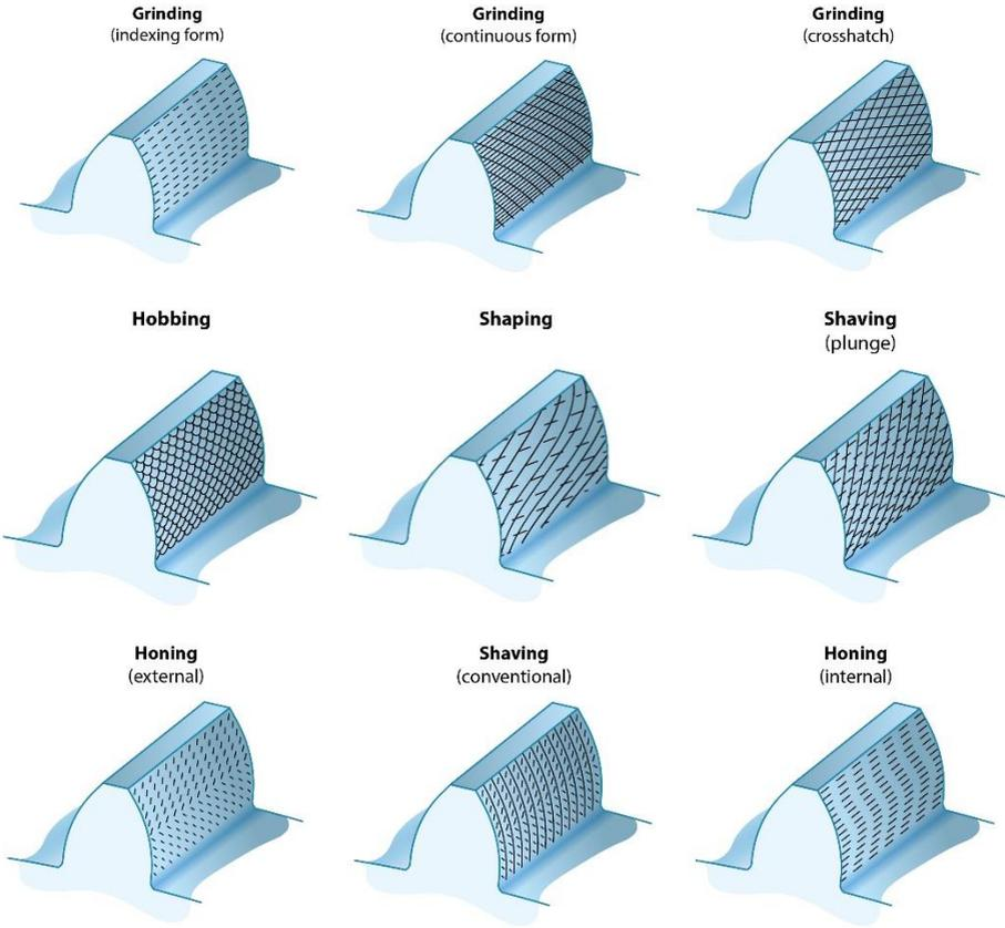
**Figure 6.** Common gear manufacturing processes and lay directions.
