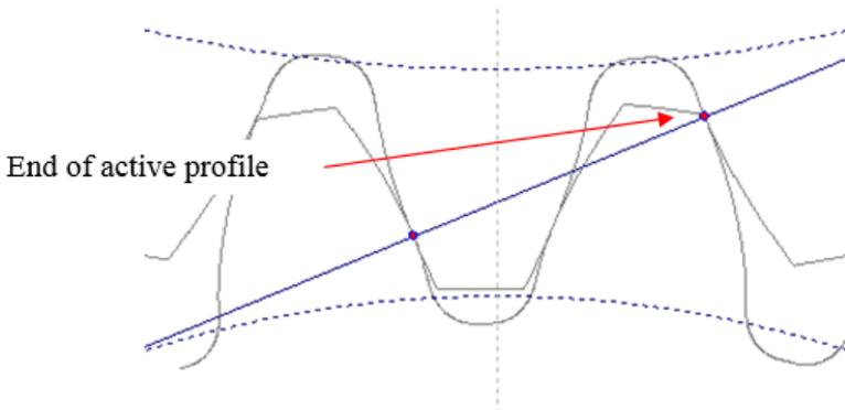
**Figure 4.** Gear positions at the end of active profile. The upper gear has a lower rolling velocity than the lower gear at the end of the active profile (EAP), again leading to a sliding action.
