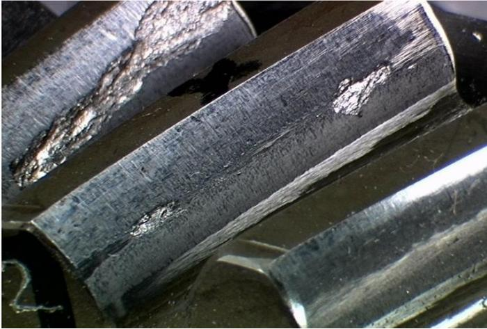
*Figure 8. Macro-pitting fatigue damage on gear teeth.*
