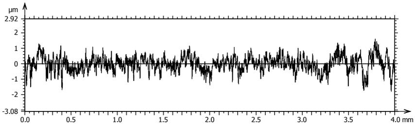
**Figure 22.** The roughness profile of a section of a gear flank, with an  $Ra$  of  $0.41\ \mu\text{m}$ .
