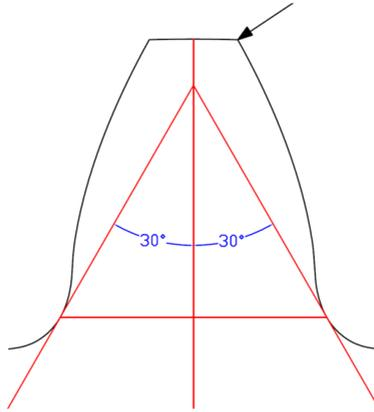
**Figure 10.**  $30^\circ$  tangent position for root fillet roughness measurement at the predicted region of maximum bending stress in BS ISO 6336-3 [16]. The arrow is the applied load.
