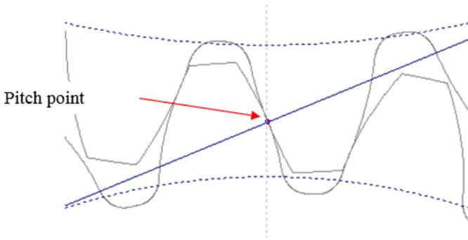
**Figure 3.** Gear positions at the pitch point, which lies on the line between the two gears where sliding speed is zero. The action is purely rolling as they both have the same rolling velocity at this time.
