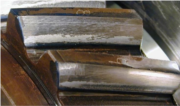
*Figure 7. Gear micro-pitting (grey staining) contact fatigue damage.*
