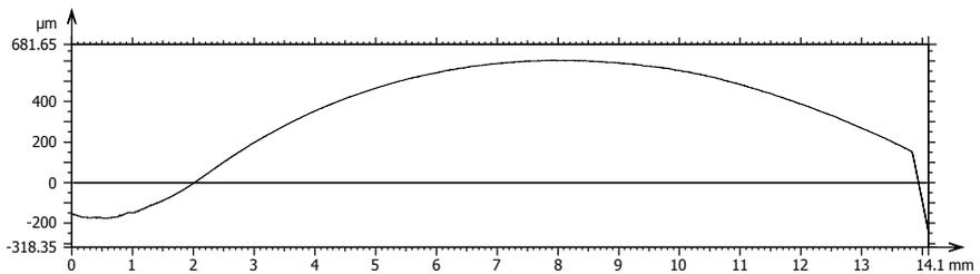
**Figure 19.** Illustration of one continuous profile measured with a general surface texture instrument from tooth root to tip.
