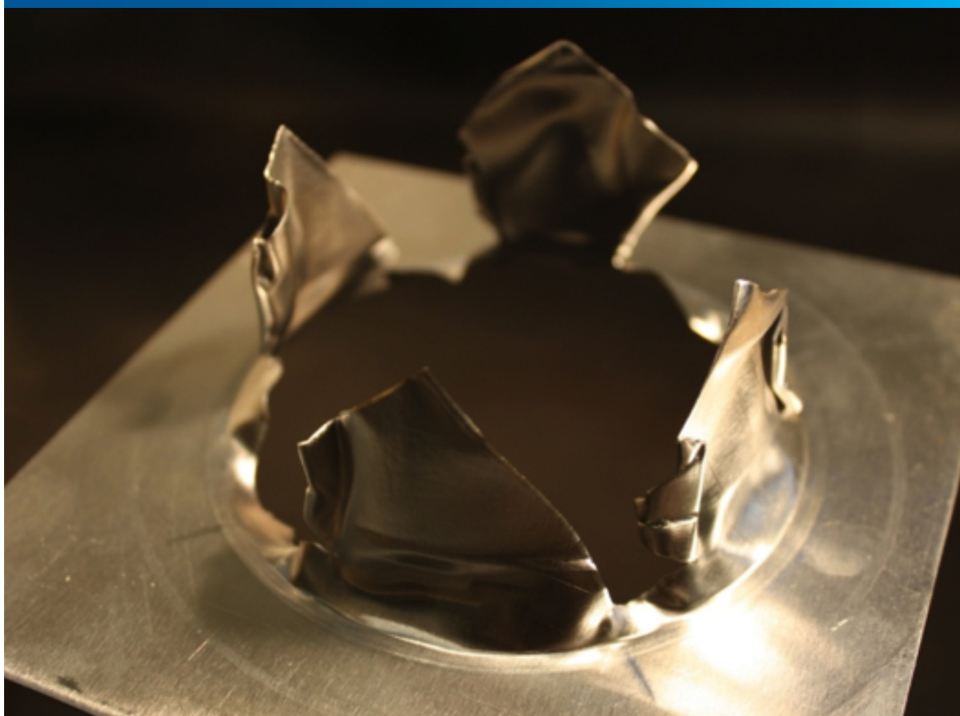
Aluminium diaphragm which was burst within the NPL shock tube.
