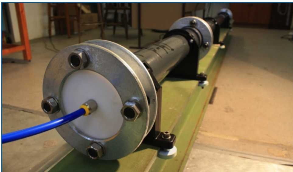
NPL 1.4 MPa shock tube, viewed from driver end.
