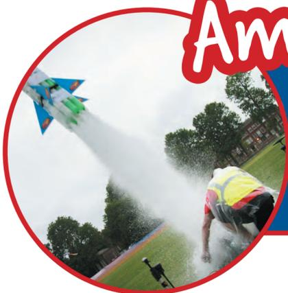
On leaving the rocket, the air expands and its heat is shared over a larger volume so it cools down, typically to  $-75^{\circ}\text{C}$ . (Yes – we checked this!)
