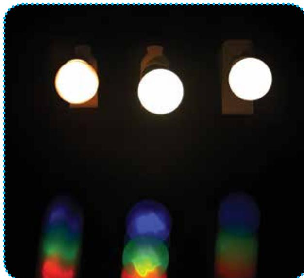
Using the fact that LEDs can detect light as well as emit it, producing an electrical signal when illuminated, NPL and the University of Surrey devised an ingenious way to measure an LED's temperature in situ.
