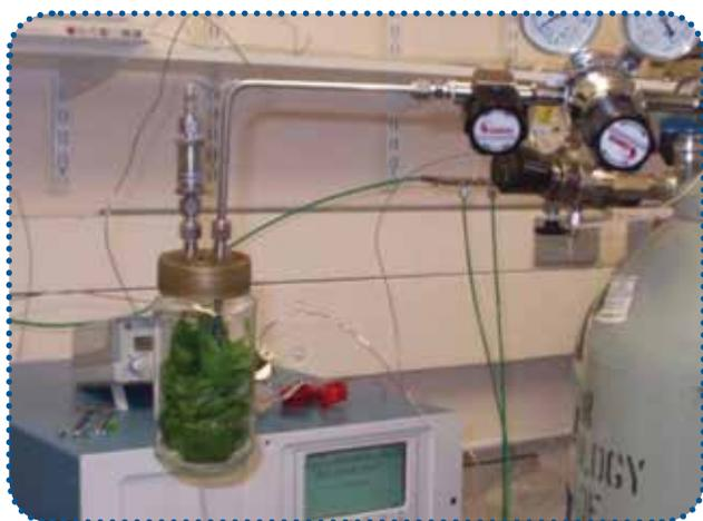
NPL had previously developed expertise in trace gas sensing techniques based on flame ionisation and it was suggested that this expertise might be applied to the detection of methane from plant sources. Through collaboration between NPL and the plant science group at the University of Sheffield a project was formulated to carry out measurements under controlled biological and metrological conditions, and to relate any methane production to photosynthesis or respiration.
