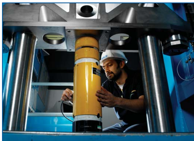
Calibrating a 4.5 MN force transducer in NPL's 1.2 MN deadweight machine
