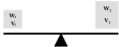
If the conventional masses are equal ( $W_1 = W_2$ ) the weights will balance in air of density  $1.2 \text{ kg m}^{-3}$
