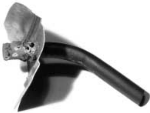
Figure 4. Accelerated corrosion of a copper tube attached to a stainless steel tank
