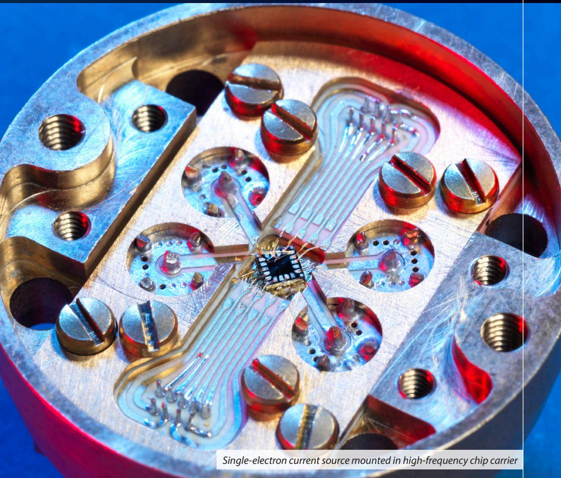
*Single-electron current source mounted in high-frequency chip carrier*
