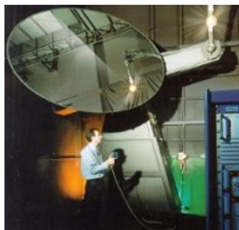
reflectance, illuminated normally by a luminous intensity standard at a measured distance. A telephotometer designed to have a response close to the  $V(\lambda)$  function measures light reflected at  $45^\circ$  to the normal. The best measurement capability is  $\pm 1.5\%$ .
