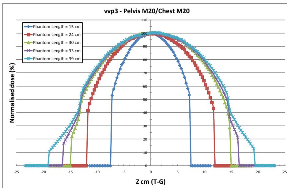
**Figure 2** MC simulated dose profiles along the central axis of the CTDI phantom at source to axis distance of 100 cm for the Pelvis M20/Chest M20 preset (vvp3) and a set of different Body Phantom lengths.
