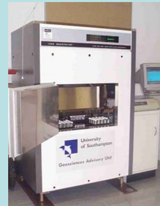
Raddec Pyrolyser and Wallac Quantalus for tritium extraction and measurement. Images courtesy of GAU
