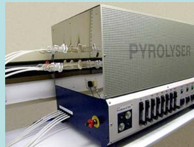
Raddec Pyrolyser and Wallac Quantalus for tritium extraction and measurement. Images courtesy of GAU
