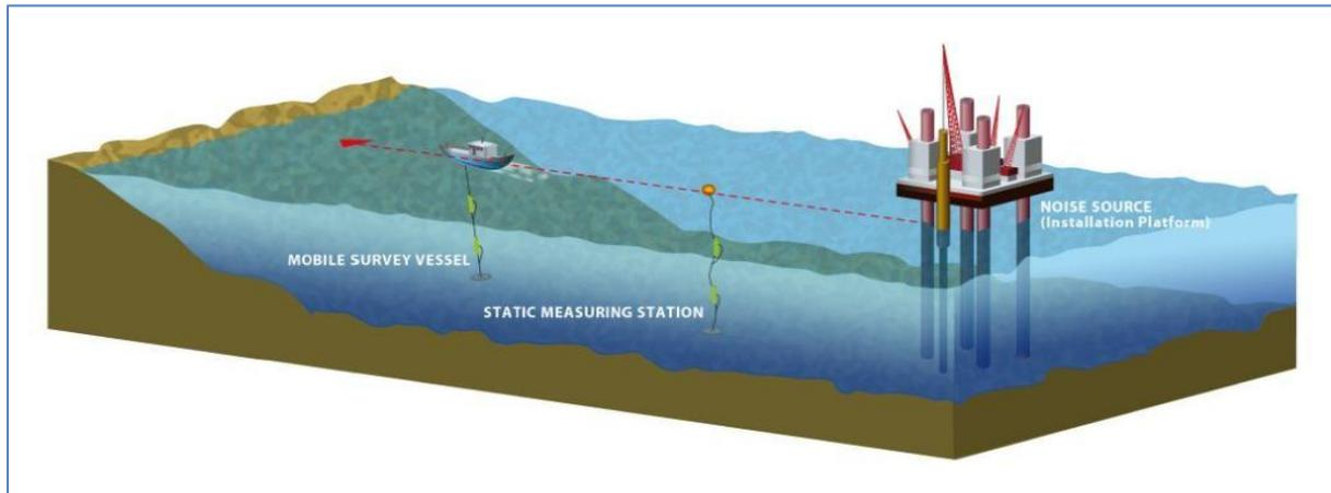
Figure 6.1: Possible deployment configuration for measuring the radiated noise in shallow water, with a static recorder and a vessel for range-dependent deployments along a transect.
