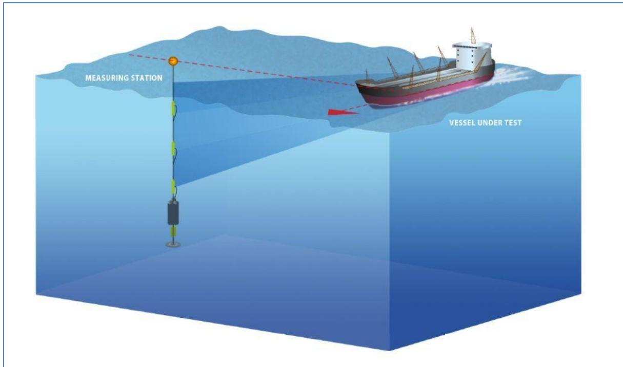
Figure 6.3: Possible deployment configuration for measuring the radiated noise in deeper water, with a hydrophones and recorder deployed from the surface. Note that the diagram is not to scale.
