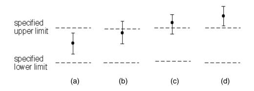
**Figure 7.** Four cases of how a measurement result and its uncertainty may lie relative to the limits of a stated specification. (Similarly, an uncertainty may overlap the lower limit of a specification.)
