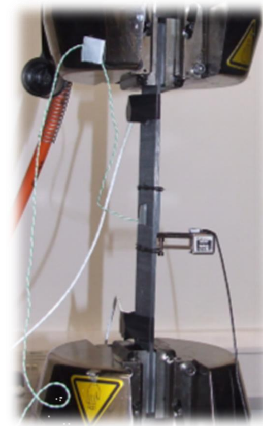
Linear location of damage using AE
