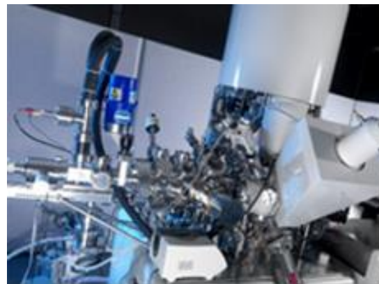
Figure 3 NPL’s X-ray photoelectron spectroscopy (XPS) instrument, used to characterise the surface chemistry of graphene
